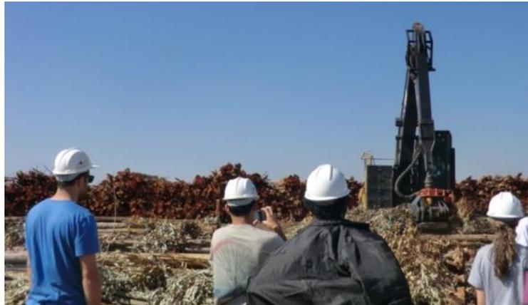
Figure 19 Mechanized feller/buncher working in a “cut-to-length” harvest system
