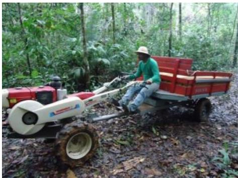
Figure 23 Micro-tractors used to forward pre-processed timber from site to access roads
