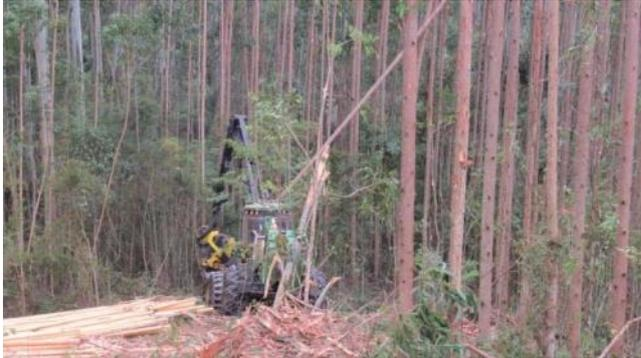
Figure 13 Harvester cutting, debarking and sectioning young *Eucalyptus* logs at a slope area
