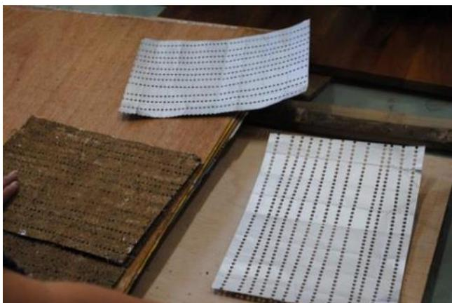
Figure 26 Bamboo ply panels with tetra-pak layer
